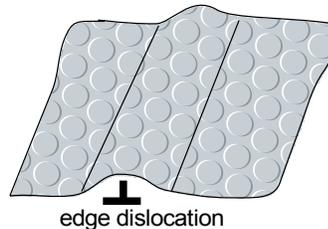
Move a wrinkle across the floor. (This represents the breaking of a row of atomic bonds in the plane.)
