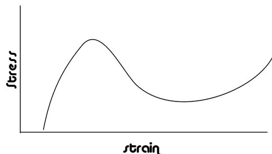
In elastomers, the polymer chains are highly kinked and twisted. With tension, they simply uncoil and align. Here, only stretching of the polymeric chains takes place. Upon release of the stress, chains spring back into their original shape. With continued stretching, chains slide past each other and the materials begins to plastically deform.
