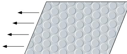
Pick up one edge of the rug, and drag it across the floor. (This represents atomic motion by breaking **all** the bonds in the plane.)
