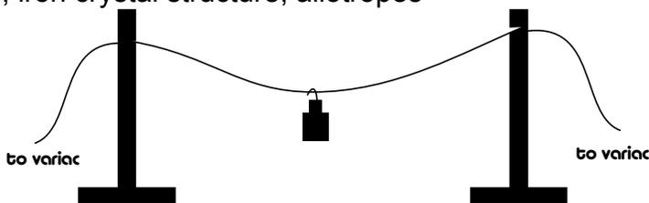
Iron has three forms (or allotropes). When heated it changes from BCC to FCC to BCC. FCC is closed packed and has a lower specific volume than BCC. So with heating, the wire lengthens, gets taut and lengthens again.
